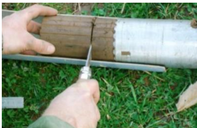
Figure 23. Separation of the soil horizons of the collected core
