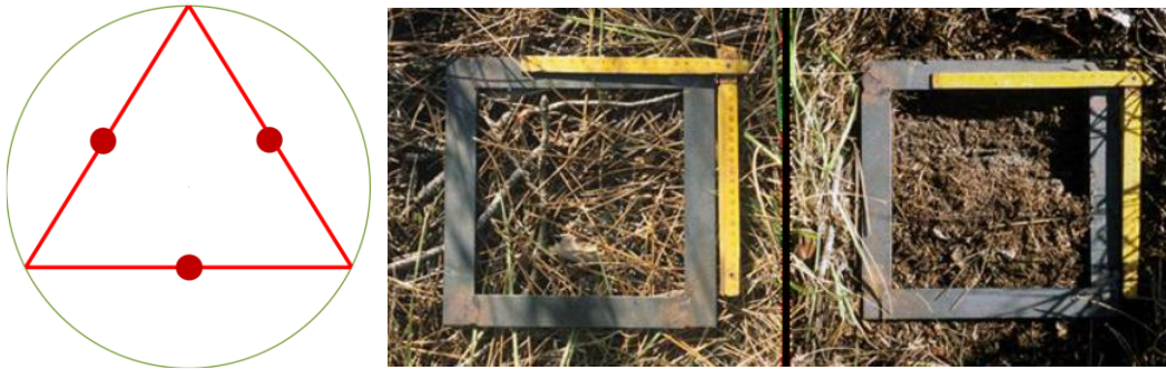
Figure 21. Litter and soil sampling scheme: red dots indicate sampling points (approximately midway along each transect). On the right is an example of litter sampling in a coniferous forest.
